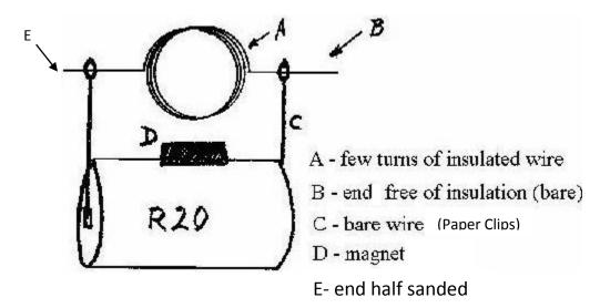
7) **COMMON ISSUESS:** You may have to give it a gentle push to get it started, but it should begin to spin rapidly. If it doesn't spin, check to make sure that all of the insulation has been removed from the wire ends, and one side is half sanded. If it spins erratically, make sure that the tails on the coil are centered on the sides of the coil.
