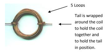
**NOTE**: Be sure to center the two tails on either side of the coil. Balance is important.
