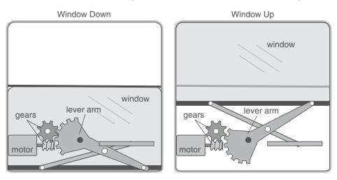
Motors for other electrical devices cause objects to move in different ways through an assembly of gears and other parts connected to a spinning axle. For example:
