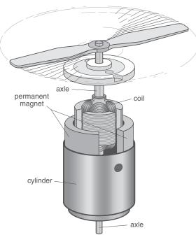
**1.** For the electromagnetic interaction in a spinning fan motor like the one shown, what are the interacting objects?
